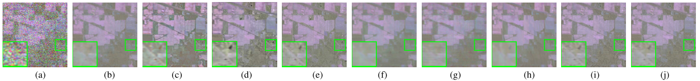
Fig. 9. Denoising results of real Indian pines dataset. The false color image is composed by bands (R: 220, G: 150, and B: 109). (a) Noisy. (b) LRTV. (c) LSSTV. (d) WSNM. (e) NMoG. (f) LRTDTV. (g) TLR-SSTV. (h) LRTDGS. (i) FGSLR 2/3 . (j) FGSLR 1/2 .
